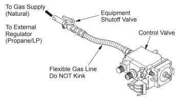
Figure 32 - Connecting Flexible Gas Line to Millivolt Valve
